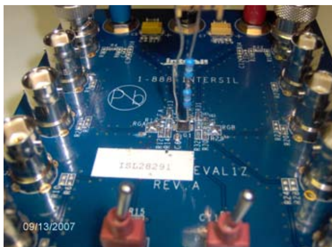
FIGURE 8. IMPROVED ANTENNA DESIGN TO EVALUATE RADIATED INTERFERENCE
